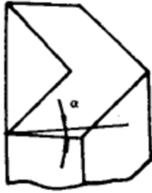
Fig. 2. Cross-sectional view of V-shaped seal ring.
