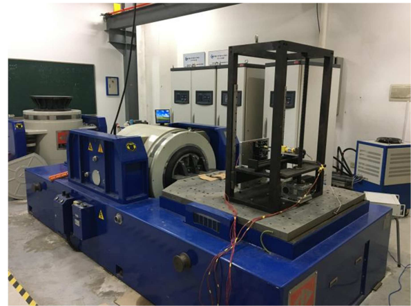
Figure 4. Vibration test system for low voltage electrical apparatus.
